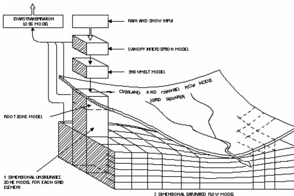
Figure 20. Schematic presentation of the SHE modelling system – image not to scale.
