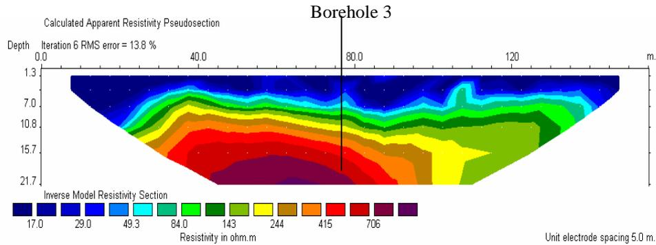
Figure 16. Electrical resistivity line. Location: study polder, about 100 m from the pump house, parallel to the embankment. Resistivity in ohm-m on the colour bar from 17.0 to 706. Horizontal interval 5m; vertical scale from 0.0 to 21.7m. Unit electrode spacing 5m.
