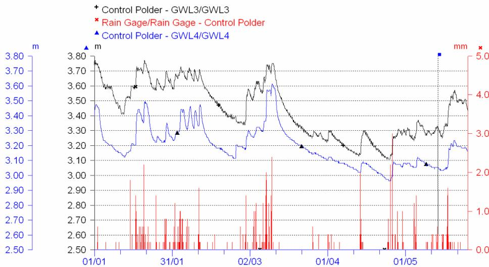
Figure 9. Hydras 3 Multiple Graphic: Rain Gauge (RG3) and two Ground Water Level Gauges (GWL3, GWL4) located in the Control Polder. Rainfall quantities in mm on the right-hand scale. Groundwater levels in m on the left-hand scale with an interval of 0.1m. Period: 01/01/2003-25/05/2003.
