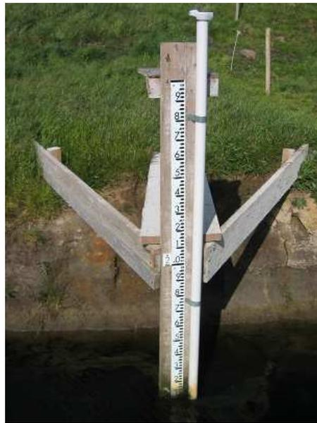
Figure 6. OTT Orphimedes water level gauge.
