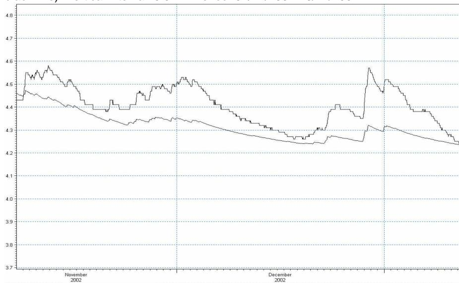
Figure 22. Ground Water level measured (GWL8-upper line) and calculated (Mike 11/SHE result file - lower line) Period: 01/11/2002-15/01/2003. Vertical interval 0.1m.
