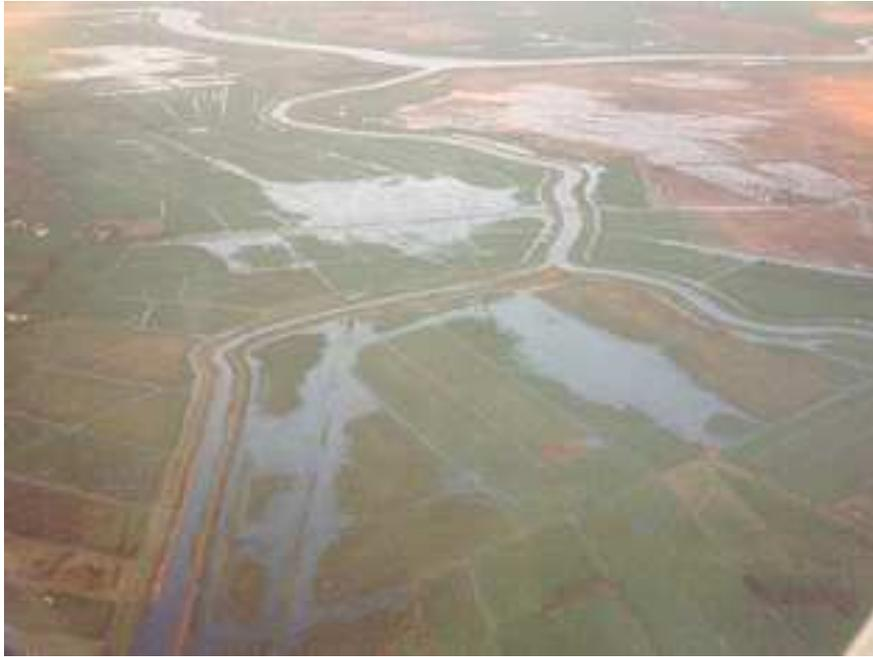
Figure 5. This photograph shows the overtopping of back-drains and land-drains in the lowlands of the Lower Feale catchment. (Office of Public Works, 1998).
