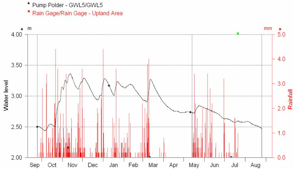
Figure 10. Hydras Multiple Graphic: Rain Gauge (RG4, red) and Ground Water Level Gauge in the Pump Polder (GWL5, black). Period: 09/2002-09/2003
