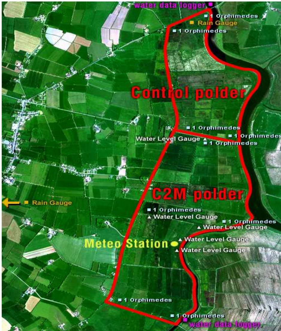
Figure 7. RGB image of the two polders showing instrument location. The upland area to the left provides rainfall-runoff into both polders.
