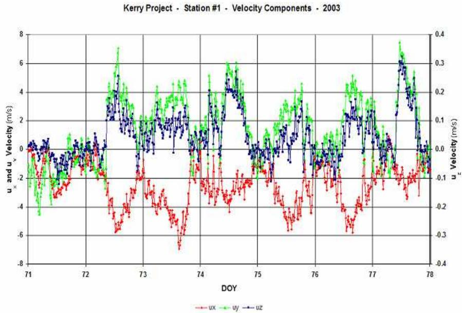
Figure 13. Velocity components  $u_x$  (red) and  $u_y$  (green): left-hand scale in units of 2 m/s. Velocity component  $u_z$  (blue): right-hand scale in units of 0.1 m/s. Components in the x, y and z directions recorded by the Eddy Correlation station. Period: 11/03/2003 – 18/03/2003: DOY – days of the year.
