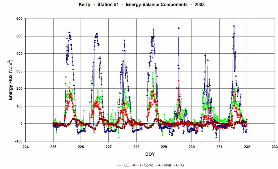
Figure 14. Energy fluxes recorded from the eddy correlation station. Period: 02/07/2003 – 08/07/2003 – DOY days of the year. Rnet (blue) is net radiation flux; LE (green) and H (red) are latent and sensible heat fluxes respectively; G (brown) is the soil heat flux. All units are Watts per square meter. Vertical interval is  $100W/m^2$ .
