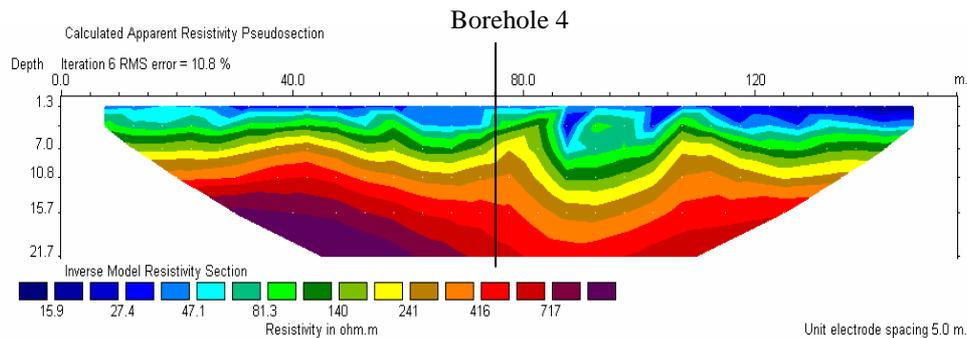
Figure 17. Electrical resistivity line. Location: study polder, 1400 m from the pump house, parallel to the embankment. Resistivity in ohm-m on the colour bar from 15.9 to 717. Horizontal interval 5m; vertical scale from 0.0 to 21.7m. Unit electrode spacing 5m.
