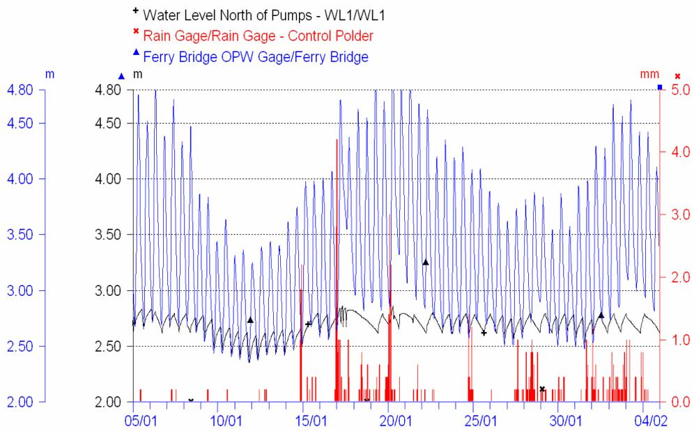
Figure 11. Hydras 3 Multiple Graphic: Rain Gauge (RG3) and two Water Level Gauges (Ferry Bridge-OPW and WL1). Period: 05/01/2003-05/02/2003.
