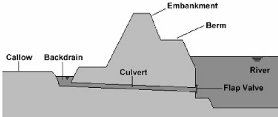
Figure 2. Cross section of embankment showing sluiced culvert link between back-drain and main embanked river.
