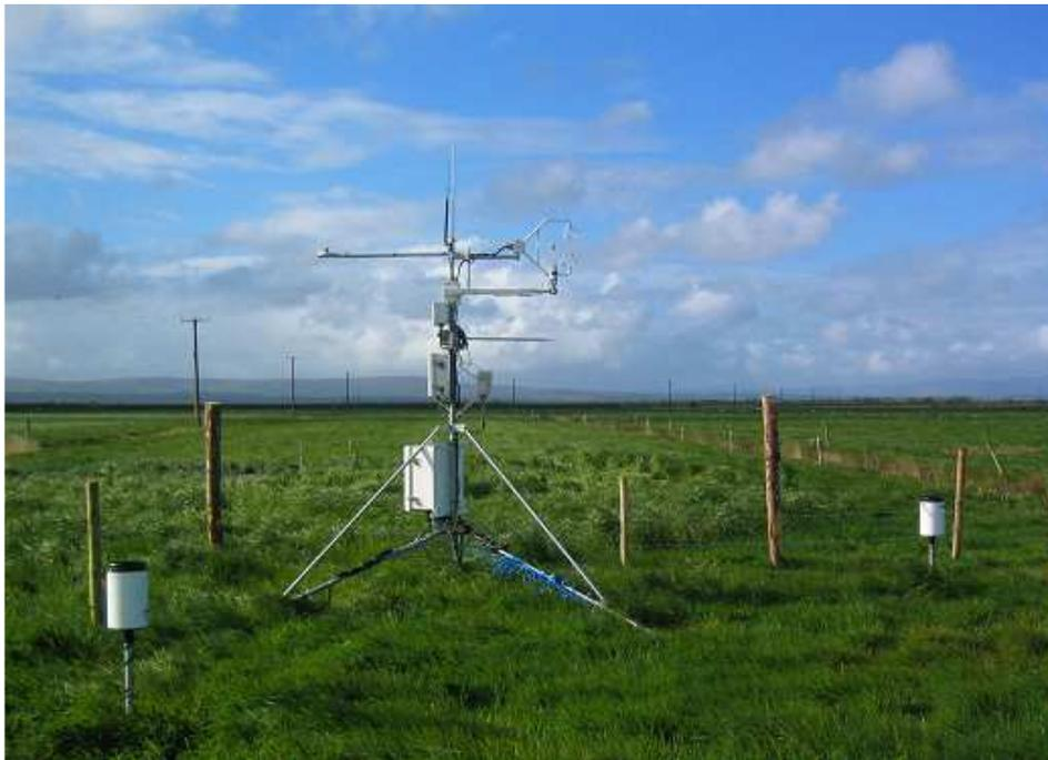
Figure 8. Eddy-correlation SVAT (soil, vegetation, atmosphere) station.
