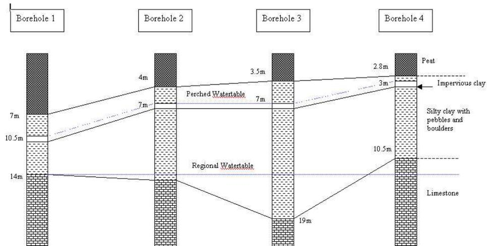
Figure 15. Boreholes logs from the study polder. Borehole logs 1 and 2 were recorded from chippings. Borehole logs 3 and 4 were recorded from core samples. The positions of the perched watertable and associated impervious clay were inferred from borehole water strikes and electrical resistivity cross-sections.
