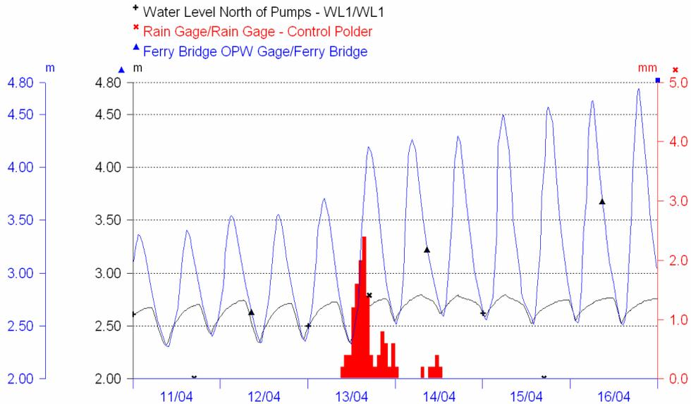
Figure 12. Hydras 3 Multiple Graphic: Rain Gauge (RG3-red) and Water Level Gauges [Ferry Bridge-blue and WL1-black]. Period: 11/04/2003-17/04/2003.
