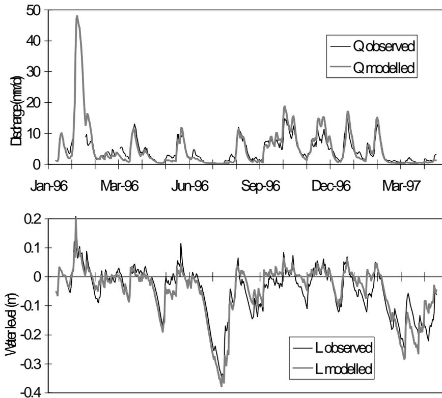
Figure 3. Modelled and observed discharges (Q) and water levels (L) for the Jemoreng catchment.
