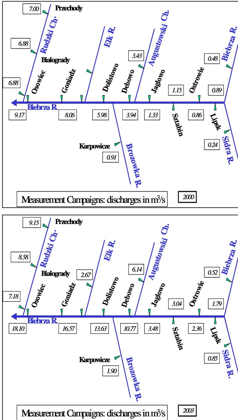
Figure 5: Discharge measurement in 2000 and 2003
